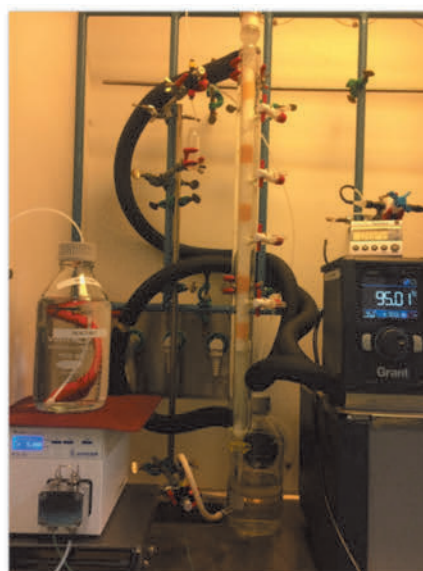
Modeling results of the autocatalytic hydrolysis of inulin in a batch reactor and the continuous reactor setup with het. catalyst.
