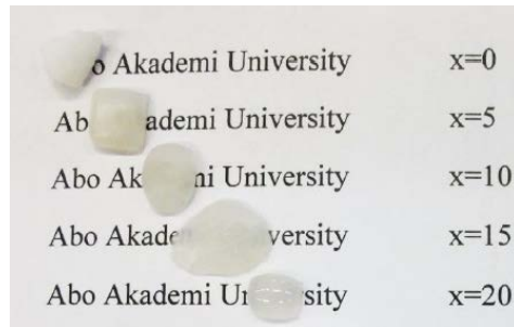
Left: 3D porous, robocasted bioactive glass-ceramic tissue engineering scaffolds (S. Eqtesadi). Right: Gradual change from opaque ( x = 0 ) to slightly translucent ( x = 20 ) appearance of thermally treated optical glasses (S. Cui)
