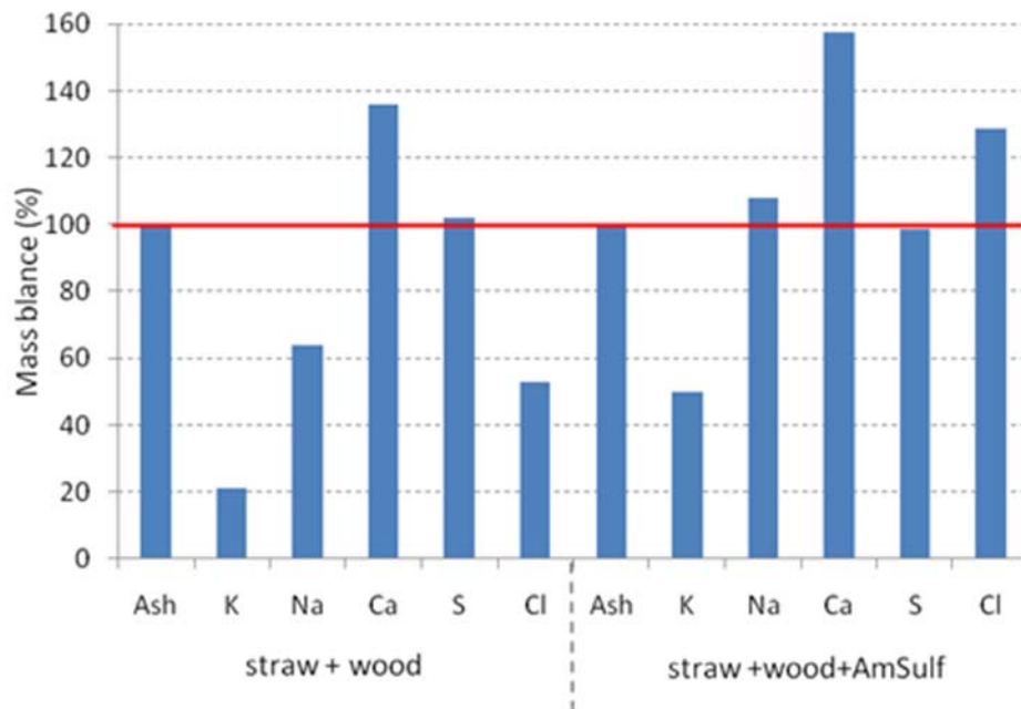
Figure 2. Mass balance of ash and different element in the experiments of day 1 (straw + wood) and day 2 (straw + wood + AmSulf).
