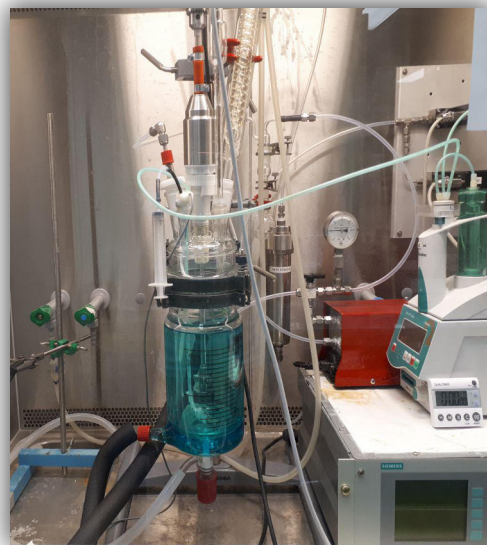
Experimental device for pharmaceuticals destruction: principally and in reality (S. Saeid, P. Tolvanen, k. Eränen).
