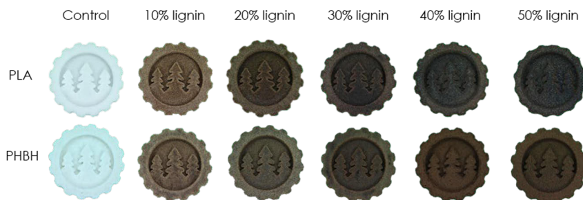
Figure 2. Powder-based PBF printed samples with various lignin implementation contents.
