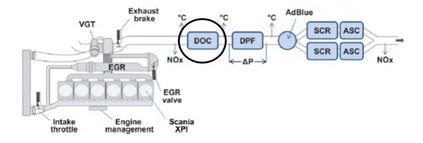
DOC Oxidizes hydrocarbons and CO into  $CO_2$  and  $H_2O$
