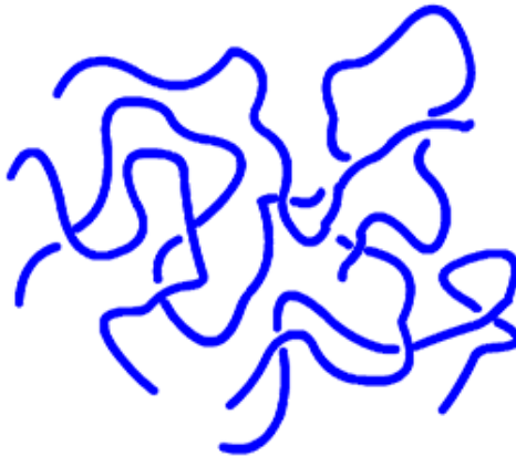
b) First step: a swollen gel in solvent
