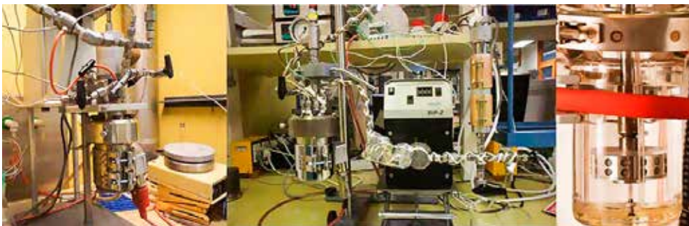
Sample wood processing with SILs. 1) Classical batch reactor to 2) loop reactor and 3) 'SpinChem' reactor
