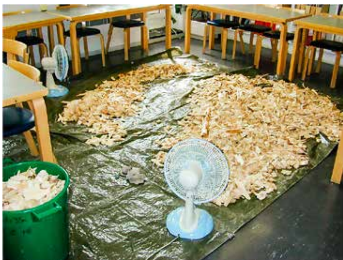
Drying of industrial oversized chips for later recovery of pinosylvins in the PINOBIO project
