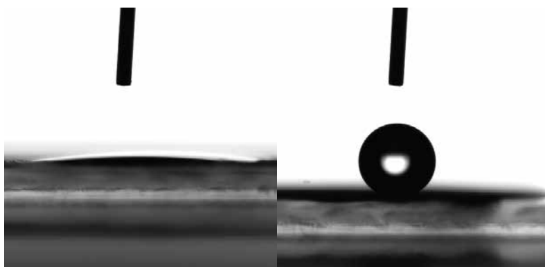
Water contact angles of polyazulene films pretreated for 10 min at 1.0 V (left) and -0.4 V (right)
