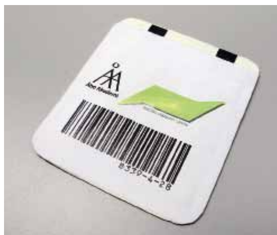
BioBattery prototype consisting of two serially connected cells
