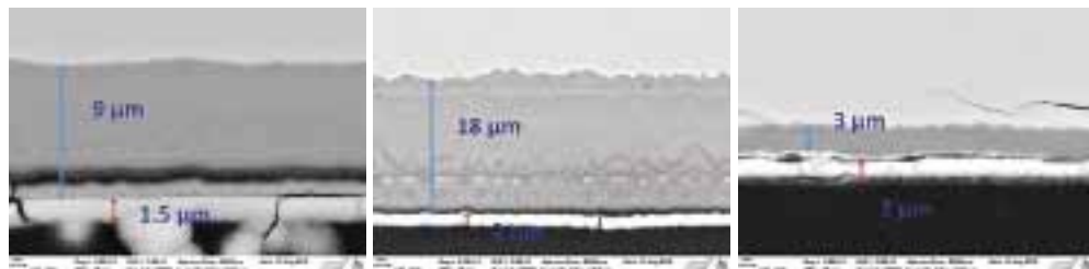
SEM images of cross-sections of bioactive glass S53P4 at 168 immersion in Simulated Body Fluid (left), Tris buffer (middle), and Sodium Phosphate Buffered Saline (right)
