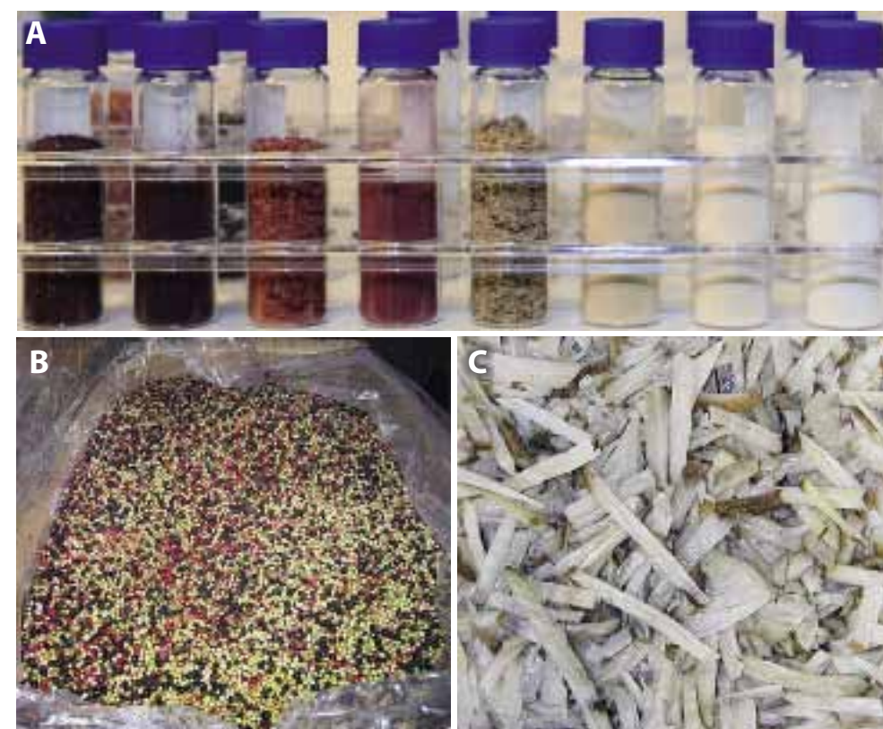
Figures A – C: Examples of side stream raw materials to be used in the project A) From left: dried berry press cake fractions. The lighter materials on the right are untreated and ground bran B) Low quality and un-matured berries to be discarded C) Beet pulp cossettes
