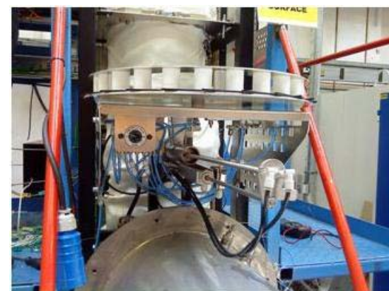
New fuel feeding system and modified grate
