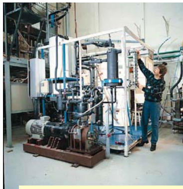
50 kW CO 2 hot water heat pump, prototype
