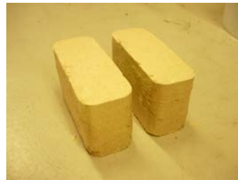
large blocked shaped briquettes (7-8%)
