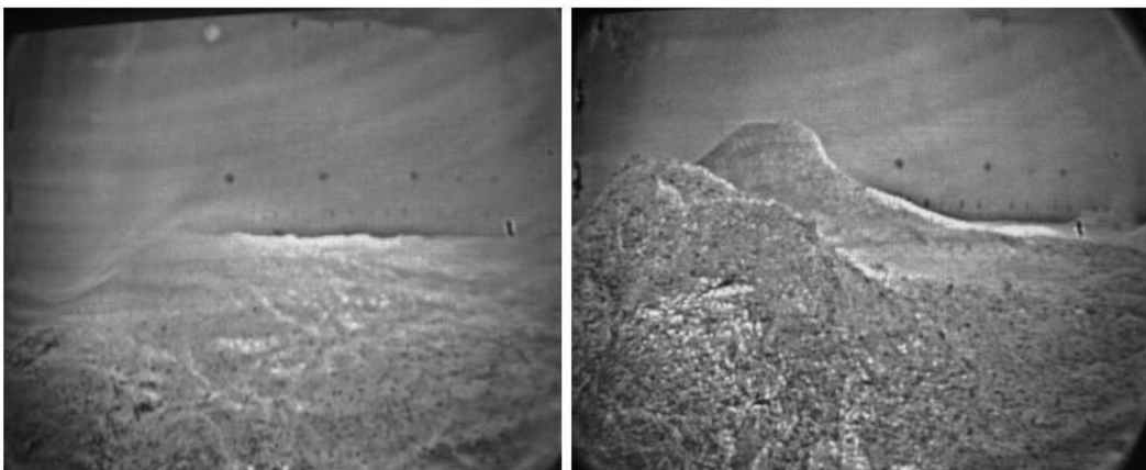
Figure 1. Pictures of the char bed during two operational modes: "low bed" (left) and "high bed" (right).
