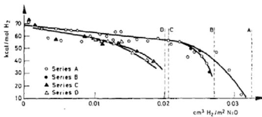
Fig. 5. Differential heats of  $H_2$  sorption by  $NiO$  at  $190^\circ$  as a function of the volume of sorbed  $H_2$ . In series A, B, C and D the catalyst contained different quantities of  $O_2$ . Dotted lines indicate maximum sorbed volumes in each series
