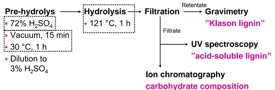
Part 1 (Hydrolysis): Alt. 1 = All moments (standard method) Alt. 2 = No vacuum/pre-heating Alt. 3 = No strong acid Alt. 4 = No hydrolysis
