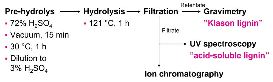
Part 1 (Hydrolysis): Alt. 1 = All moments (standard method) Alt. 2 = No vacuum/pre-heating Alt. 3 = No strong acid Alt. 4 = No hydrolysis
