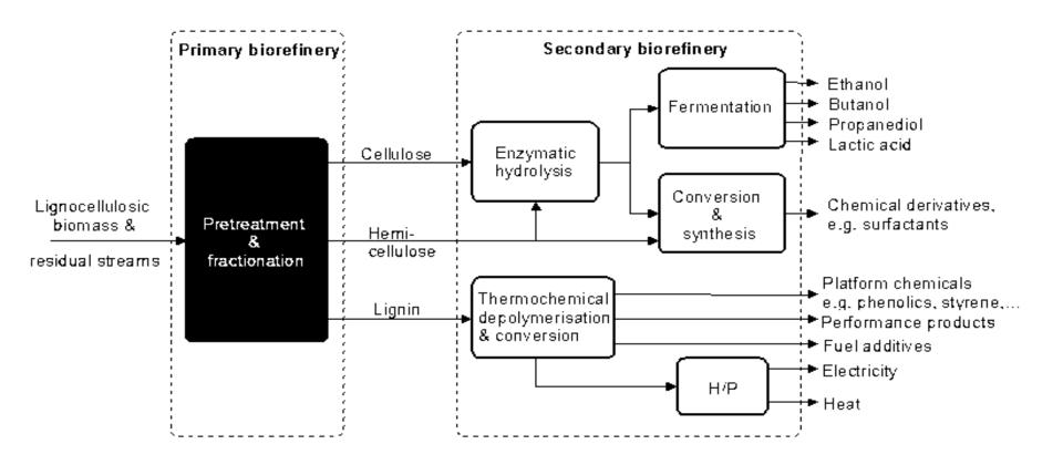
lignocellulose pretreatment to fractionate the recalcitrant lignocellulose structure; enzymatic hydrolysis of the isolated cellulose moiety, by which cellulases hydrolyze reactive intermediates to fermentable sugars; and fermentation, which produces cellulosic ethanol or other bio-based chemicals
