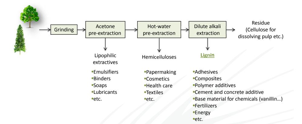
Due to its phenolic structure, lignin has great potential in different areas. Extraction from wood using pressurised hot water with addition of alkali is a promising way to obtain new, more reactive types of lignin for future applications.
