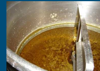
2 nd Delignification 6 wt% NaOH, 2h, 90 °C
