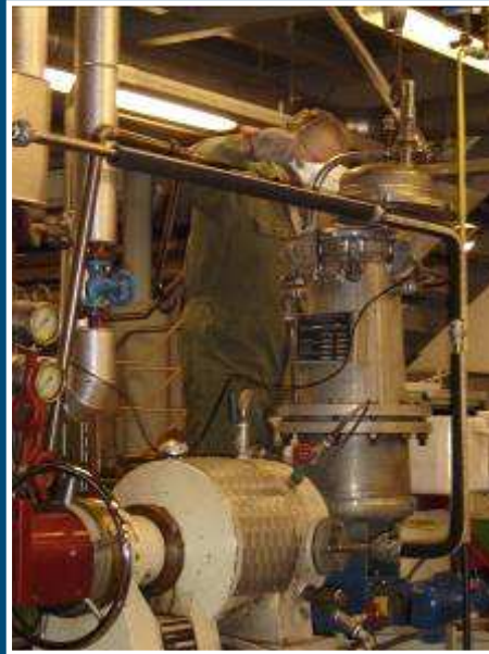
1 st Delignification Chopped wheat straw 6 wt% NaOH, 2h, 90 °C
