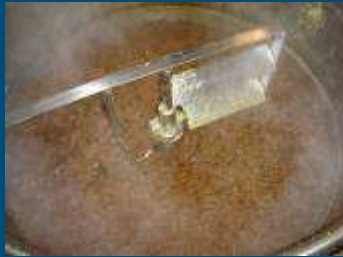
1 st Delignification Chopped wheat straw 6 wt% NaOH, 2h, 90 °C
