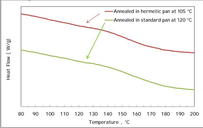
Annealing of kraft lignin at 120 °C  $\,$  in standard pan showed a Tg of 155°C Annealing of kraft lignin at 105 °C  $\,$  in a vented hermetic pan showed  $\,$  a Tg of 152°C  $\,$
