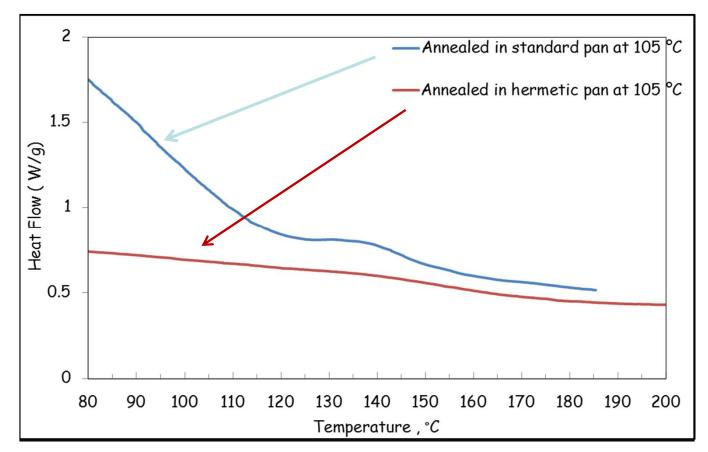
With same procedure, vented hermetic DSC pan, shows smoother data than the standard pan.
