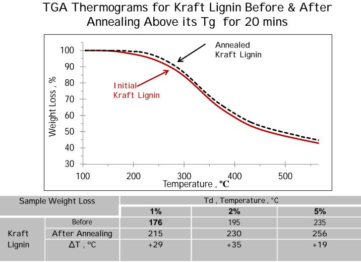
The Thermal Decomposition behavior of Kraft Lignin was changed after Annealing above its Tg It seems that annealing induces changes within the lignin structure leading to greater thermal stability.
