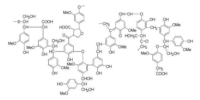
Softwood kraft lignin is highly susceptible to thermally induced reactions that cause its molecular characteristics to be severely altered. These events seriously interfere and prevent such materials from being considered as candidates for thermoplastic applications.
