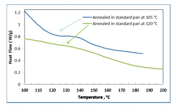
Using a standard pan shows that annealing at 120 °C is an acceptable temperature
