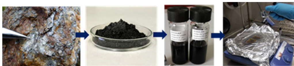
The evolution of materials from the flake graphite bearing rock sample in Haapamäki (on the left) to purified graphite powder, few-layer graphene dispersions and finally, to the spray-coated few-layer graphene films (on the right)
