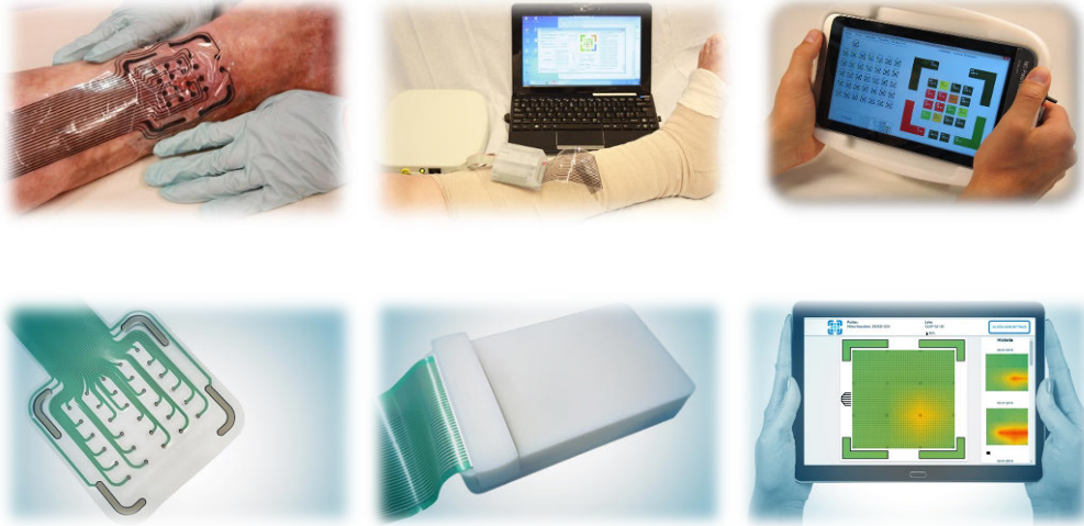
Figure 2. Upper row; the patch, the full system and the measurement device as available during clinical trial 1. Lower row; the close to final patch design, pre-production electronics and user interface. The design of the final system is not shown as market entry is expected during Q1 2021.
