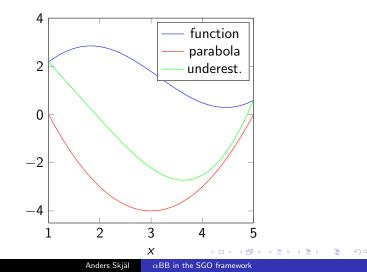
This convex underestimator can be extended to multiple dimensions. Let f be a  $C^2$  function on  $\mathbb{R}^n$ . For a large enough  $\alpha$  the function g = f + q where
